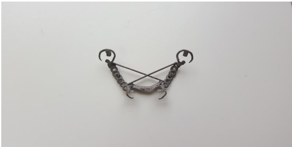
Figure2. Finished metal framework produced with the selective laser melting technique (unpolished).
